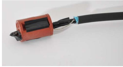
**3) Use the foil to shield the end connection.**
